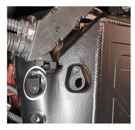
Fasten the rear bracket for the front wiring channel to the intake manifold with 1 x M5 screw included.
