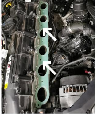
Mount 6pcs of the included sealing rings to the intake manifold flange.
