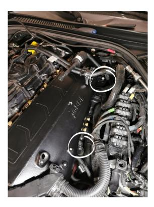
Mount the intake manifold to the two brackets with included M6 screws and spring washers.
