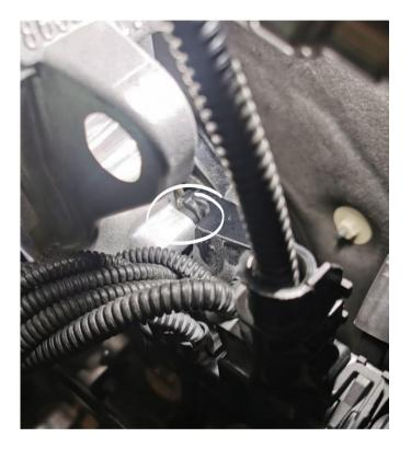
Mount the included plastic spacer between the channel and engine to move it back a bit and reinstall the T30 holding the inner wire channel. Put the outer wire channel back in position and fasten it with the 2 x E8 screws.
