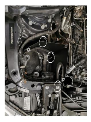
Mount the heat shield in the car and secure the front tab between the frame and core support brace. Then reinstall the snap lock and secure the back with included bolt, nut and washer.
