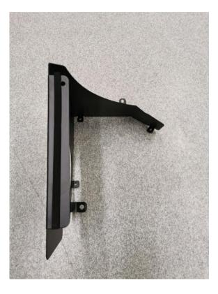
Install the included foam strip to the flat edge on the bottom of the heat shield.
