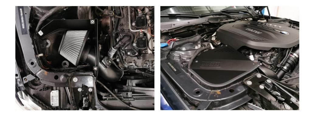
Install the air filter and secure it with the included hose clamp.
