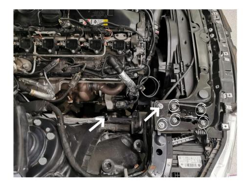
Start by disconnect the air mass meter and loosen the intake hose clamp. Then you can remove the entire filter box and intake hose together.
