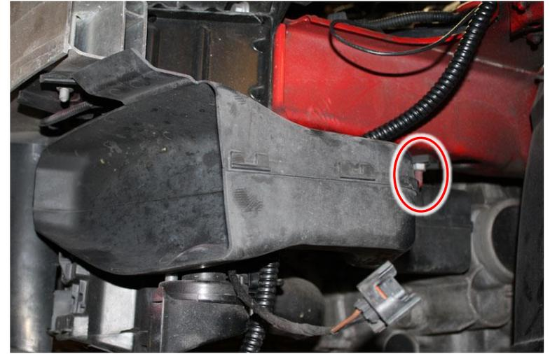
12. Remove 8x Hex 16mm screws for the two radiator bulkhead main brackets.
