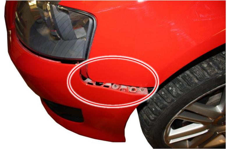
8. On cars equipped with headlight washers, clamp the headlight washer hose with a suitable tool as shown on the photo.
