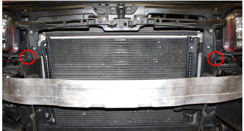
16. Gently pull the entire radiator bulkhead forward about 100mm. Let it rest in an angle like on the photo. Make sure it is not resting on the edges/corners of the front fenders!
