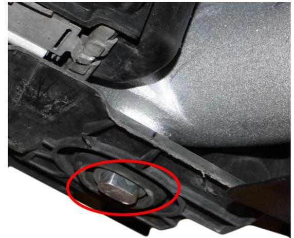
**27.** Reinstall the 2x Torx T30 for the two intercooler brackets (removed in step 15).
