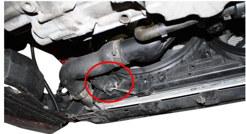
15. Remove 2x Torx T30 for the two intercooler brackets.
