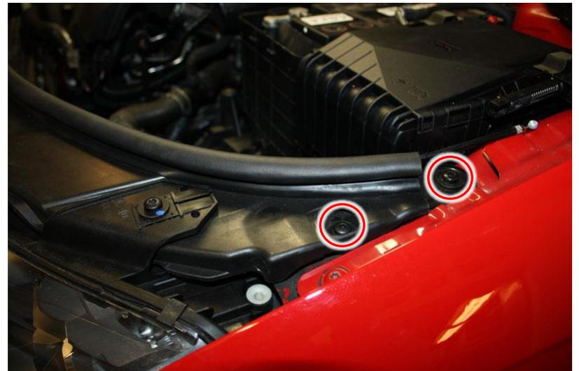
11. Remove 1x Hex 13mm nut for the air guide on the drivers side.
