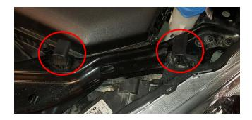
4. In the bottom of the bumper remove 3pcs plastic rivets. Press both the plastic tabs towards the middle and then gently pull it out in its collar.
