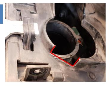
The plastic above the intercooler connection with the sensor installed to it might need to be trimmed slightly to make space for the sensor and cable. If necessary, carefully cut the plastic air guide according to picture using a metal shears.
