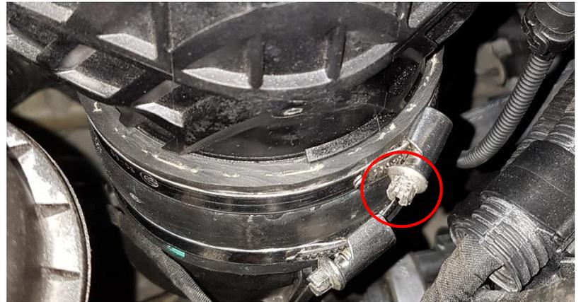
4. Use three hose pincher pliers to keep most of the coolant from draining out. Release the clips on the connectors and immediately plug the connections on the intercooler with the 21mm silicone cap.
