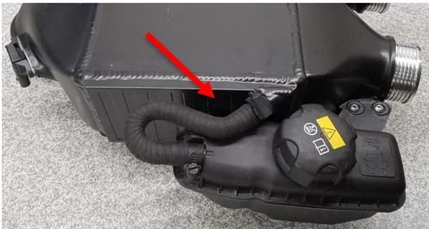
11. Remove 2x Torx T25 holding the sensor on the OEM intercooler, remove it from the intercooler and mount it on the do88 intercooler with the included 2x M5x12mm Allen screws.
