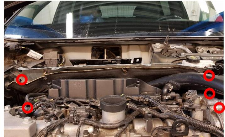
10. Remove the top section of the inlet pipe. Disconnect 4x hose clamps, vacuum line and breather hose. Gently lift pipe out of its two brackets.
