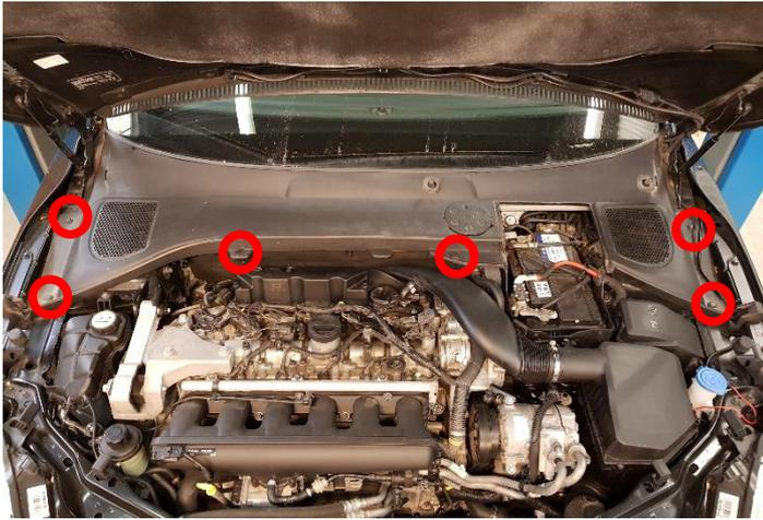
6. Remove 4x Hex 10mm plastic nuts for the firewall insulation.
