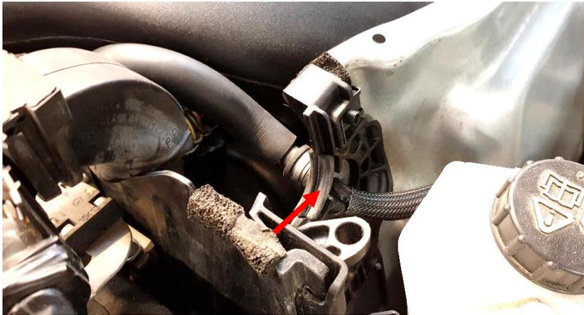
9. Remove 5x Hex 8mm screws for the firewall steel cover.
