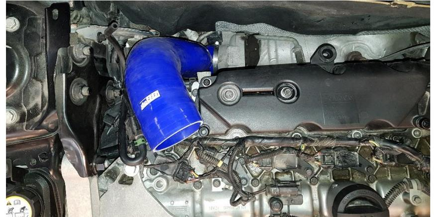
**17.** Replace the hose between solenoid and inlet pipe with the included vacuum line. Fasten the solenoid to the marked T30 Torx screw using the included cable-tie and 90deg bracket.
