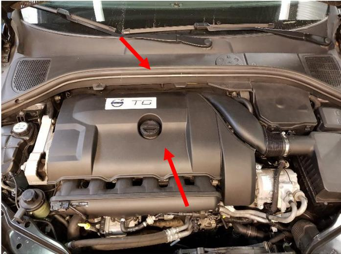
2. Remove the windshield wiper arms. Pry away the plastic cover and loosen 2x Hex 15mm nuts.
