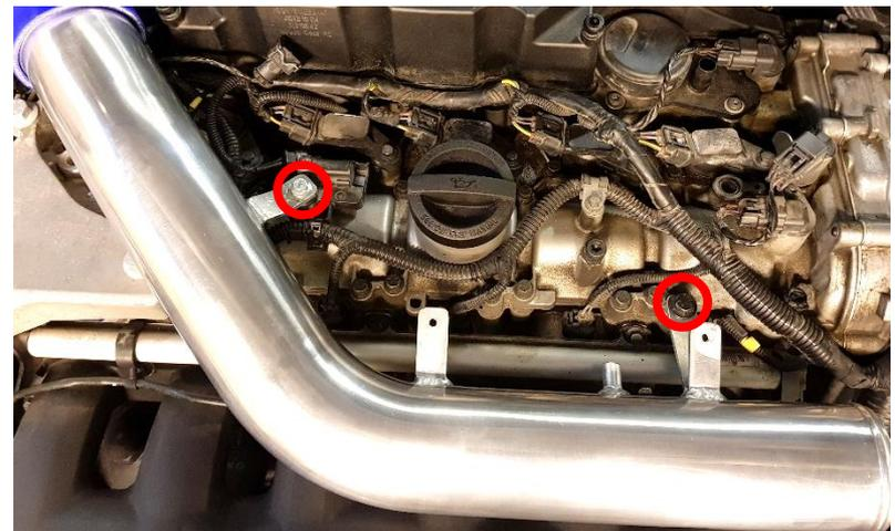
19. Check that pipe has clearance between ignition coil connector and also between pipe and the edge of the engine bracket. If you have any interference you will need to gently adjust the bracket(s). Minor deviations may occur since pipe is hand built.
