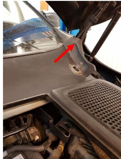
5. Remove six plastic clips and then remove the plastic cover underneath the windshield.
