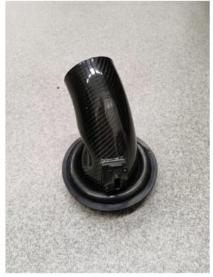
Position the plastic air duct and enter one of the included Phillips screws at a time just about 0,5-1 turn into the screw clips.
