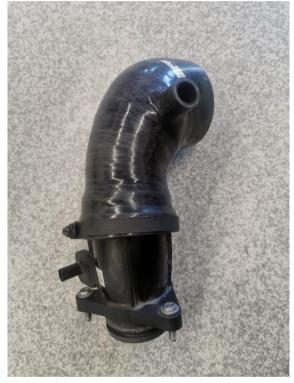
Mount the included evap adapter to the turbo inlet hose end secure with included hose clamp. Connect the evap to the adapter.
