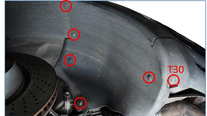
6. Remove 4pcs Torx T30 screws from the bottom of the rear bumper. Picture shows two of them, the other two are positioned in the same locations on the right hand side of the car.
