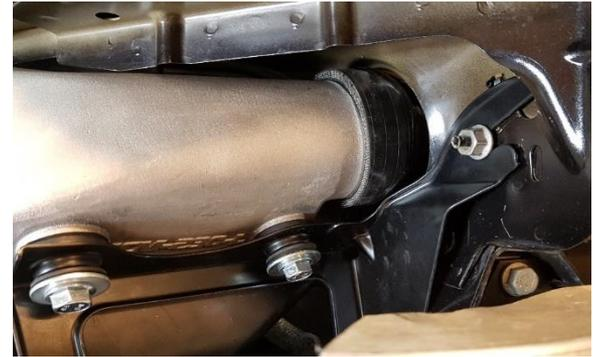
**15.** Re-install the air filter box and install the Y-pipe. Align the intercooler outlet hoses into a good position and then tighten all the hose clamps.
