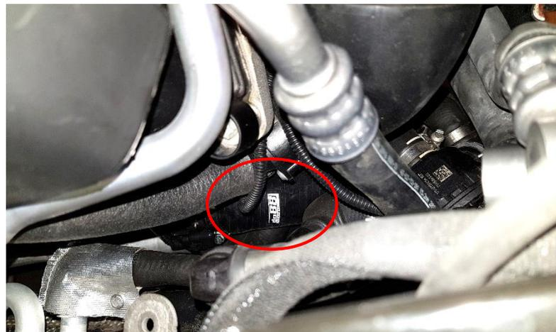
15. Now reinstall the intercooler. Before installing it put some lubrication on the connections to make the sealing slide on more easily.
