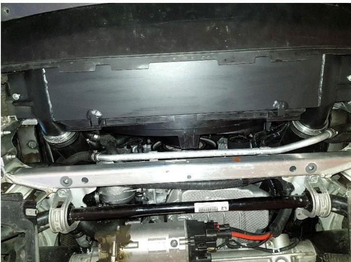
16. Now tighten the intercooler outlet hose hose clamp. Reinstall all other parts in reverse order.
