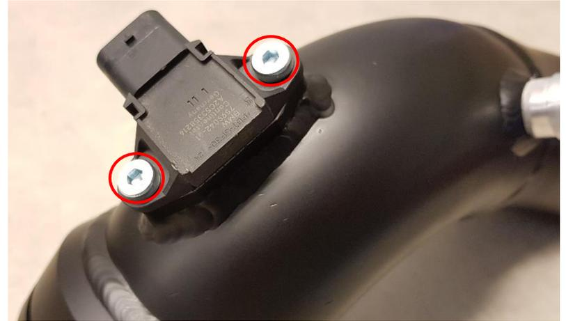
10. Remove the throttle body O-ring from the OEM pipe and install it into the do88 intercooler pipe.
