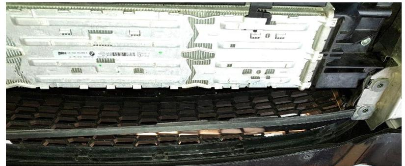
4. Remove 1x Torx T27 on each side of the intercooler then gently remove the intercooler from the car.
