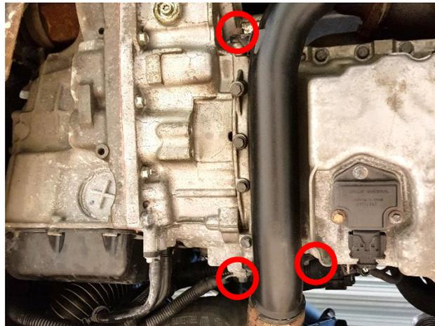
5. Remove pipe together with the hoses.
