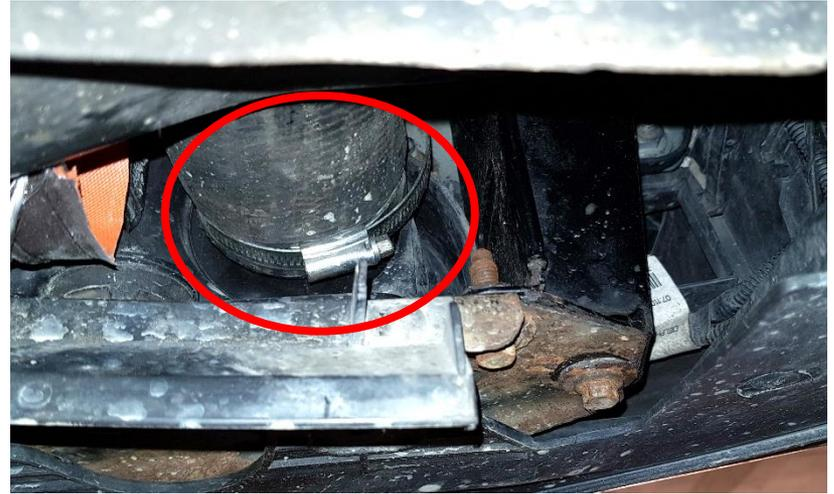
7. Loosen the hose clamp on the throttle body.
