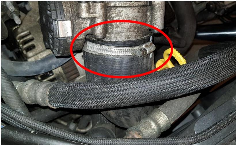
8. Remove the intercooler to throttle body hose.
