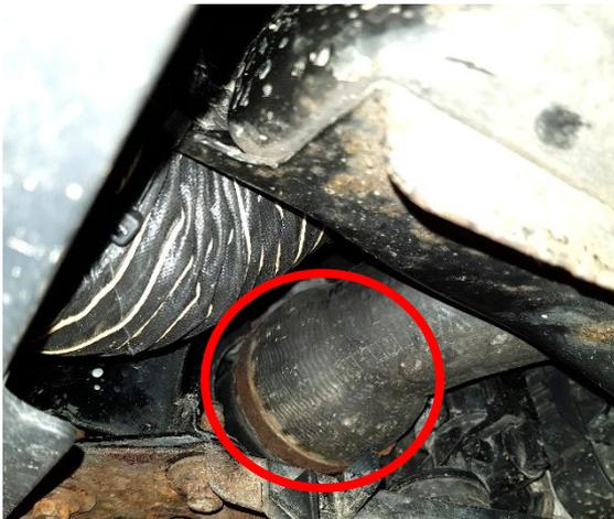
4. Remove 3x Hex 10mm screws that hold the plastic intercooler pipe.
