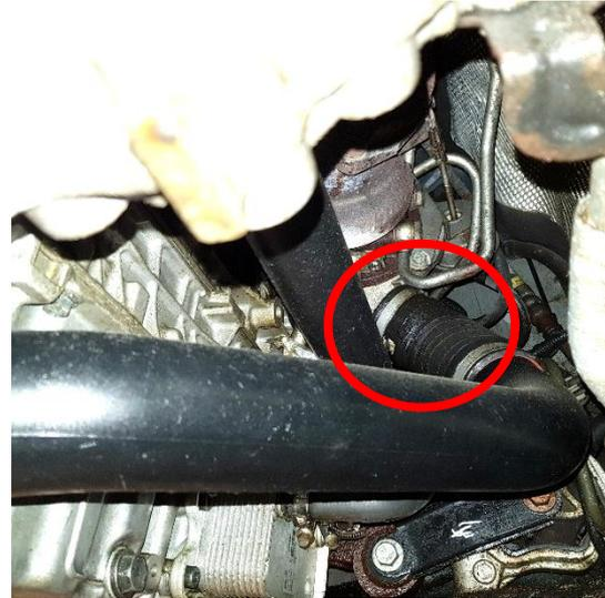
4. Loosen the hose clamp on the intercooler inlet and pull off the hose from the connection.
